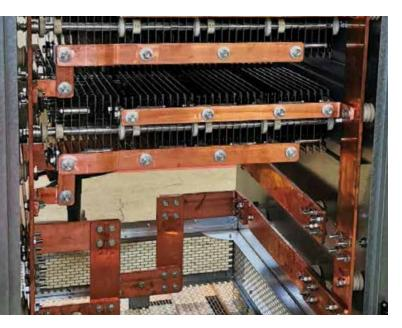
The projected performance data in the development phase of contact based and electronic switching devices, needs to be checked frequently. The demand for test resistors has risen further due to the increased importance of electro mobility. So, test resistors are necessary in order to test batteries and power packs. These battery test resistors serve to test the specified capacities and load /discharge. A number of different connections as well as some very high currents are important here.
